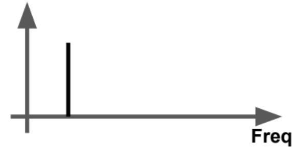
CW measurements in the frequency domain:
