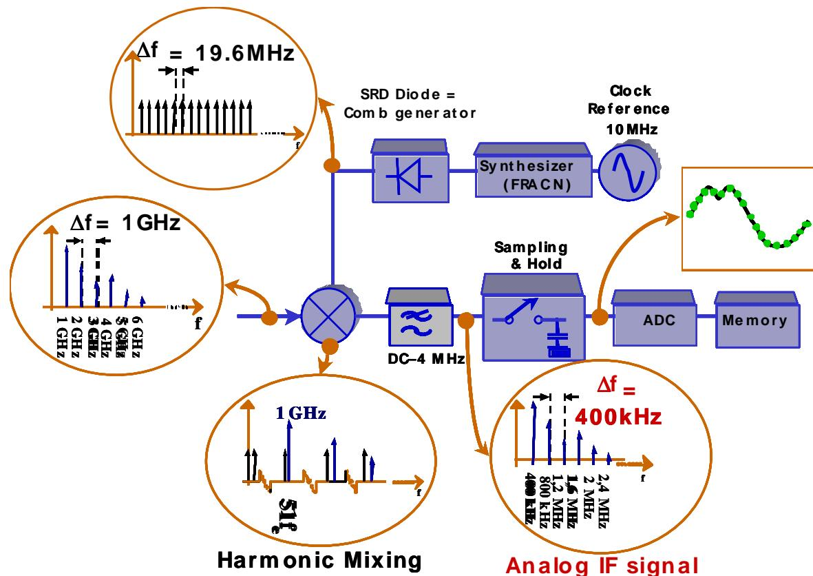
➤ Analog IF signal is an equivalent image of the analog RF signal
