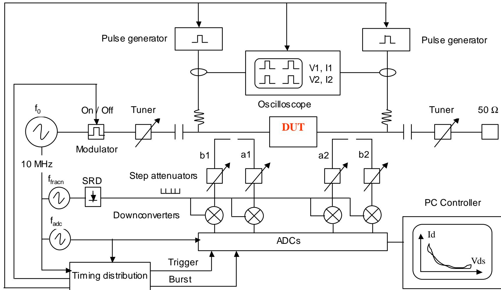
➤ All frequencies/clocks derive from the RF synthesizer high precision reference
