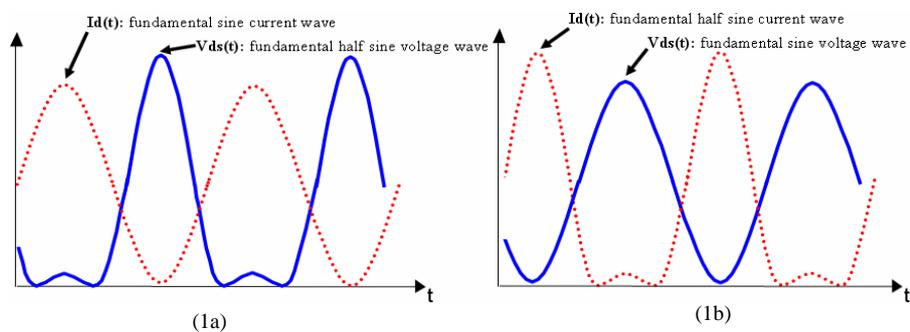
Fig. 1 Output voltage and current waveforms when an open circuit (a) or a short circuit (b) are presented at the 2<sup>nd</sup> harmonic frequency.
