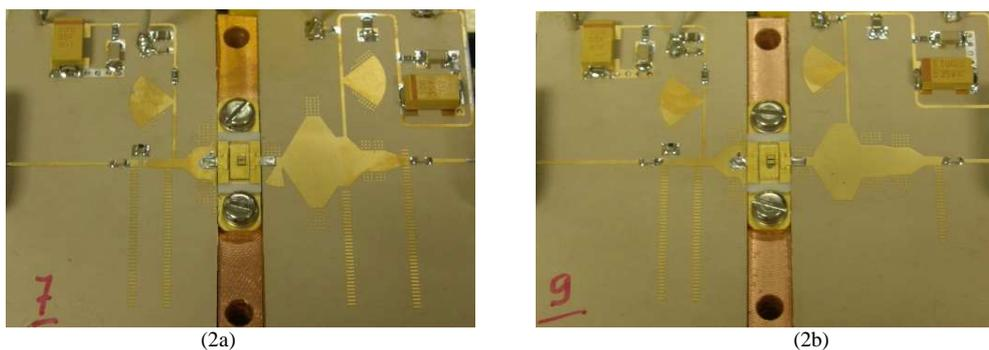
Fig. 2. Power amplifiers with optimized 2<sup>nd</sup> harmonic (a) and without optimized 2<sup>nd</sup> harmonic (b).
