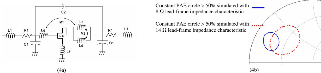
Fig. 4. Equivalent circuit of ceramic package (4.a). Constant PAE circles comparison within reference package plane for two lead-frame impedance characteristics at  $f_{\min}$  (4.b).
