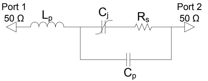
Fig. 1 Varactor diode model commonly used.
