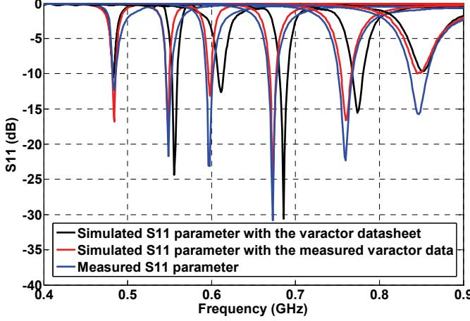
Fig. 5 Comparison between return losses.
