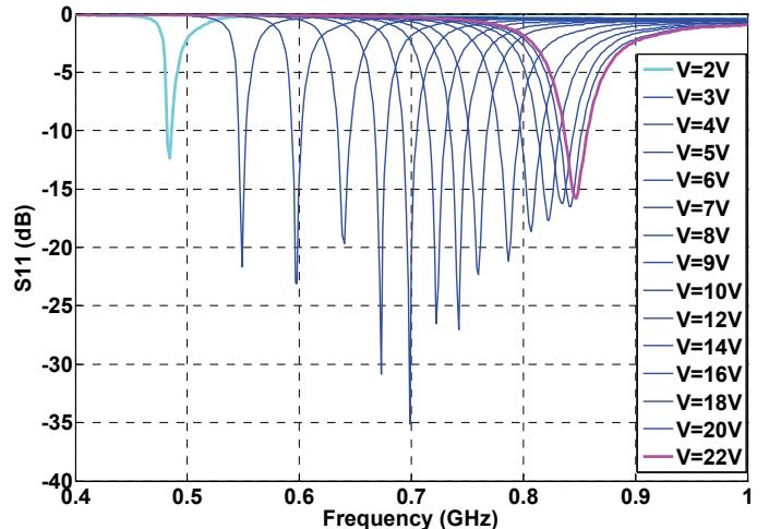
Fig. 4 Return losses for multiple polarizations of the varactor diode.
