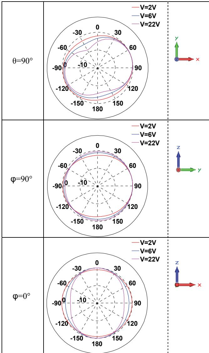
The shapes of these radiation patterns show omnidirectional patterns whatever the polarizations of the diode so, whatever the operating frequency of the antenna.
