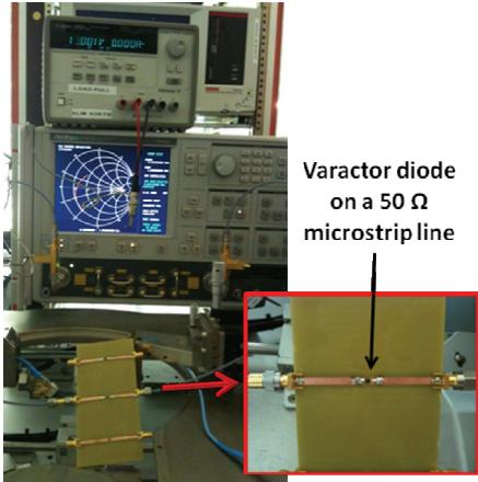
Fig. 2 Characterization of the hyperabrupt varacor diode.
